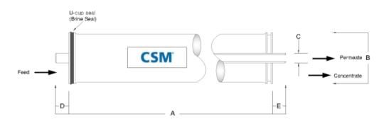
1. Each membrane element supplied with one brine seal, one interconnector (coupler) and four o-rings. 2. All RE4040 elements fit nominal 4.0 inch (101.6 mm) I.D. pressure vessels.
