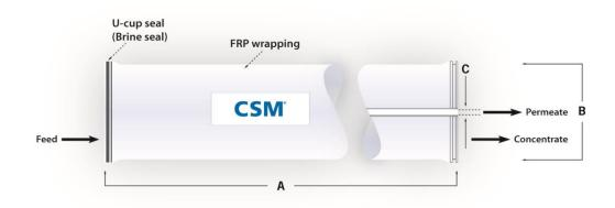
1. Each membrane element supplied with one brine seal, one interconnector (coupler) and four o-rings. 2. All RE8040 elements fit nominal 8.0 inch (203.2 mm) I.D. pressure vessels.
