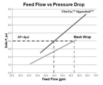
Pressure Drop versus Feed Flow for Mesh wrap and FilmTec<sup>™</sup> Hypershell<sup>™</sup> 8038 elements. FilmTec<sup>™</sup> Hypershell<sup>™</sup> has less exterior bypassing and requires approximately 30% less flow than mesh wrap for an equivalent pressure drop.
