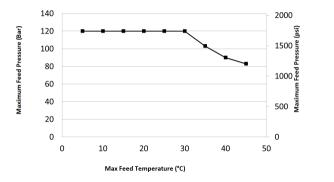
Maximum feed pressure as a function of feed temperature
